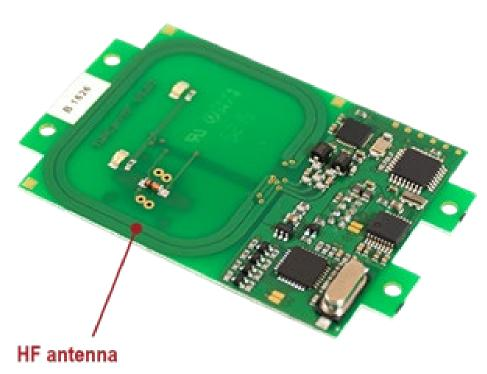
TWN3 MIFARE M - HF antenna (PCB air coil, integrated)
