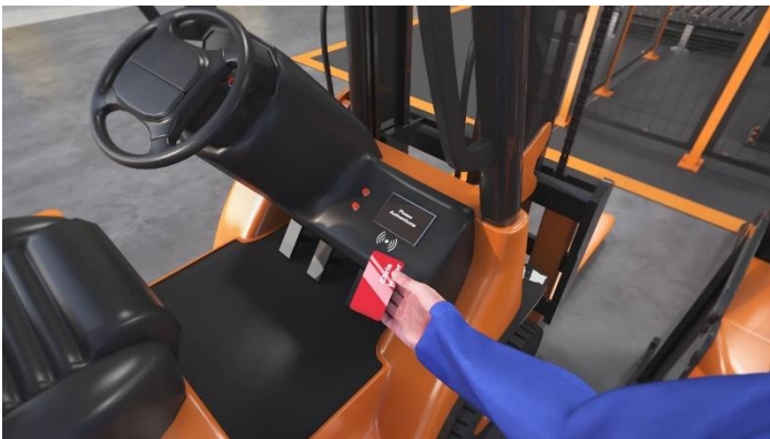
The employee ID card is generally used as an identification medium in production -but smartphones can also be used.
