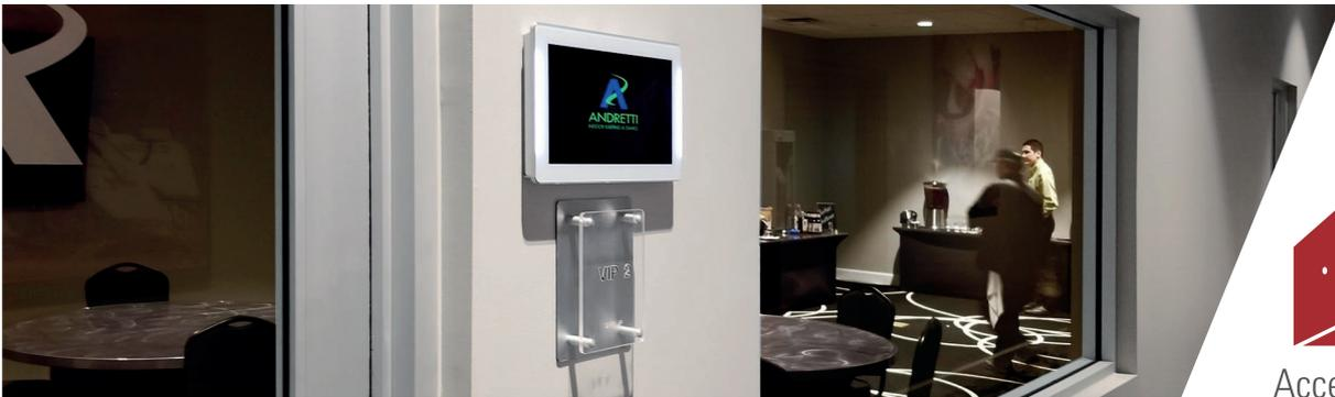
Meeting Machines integrates ELATEC's RFID TWN4 MultiTech Nano module to enable contactless meeting room check-in and control in a stylish all-in-one display.
